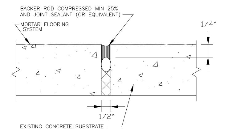
NOTE: JOINT SEALANT WIDTH TO DEPTH RATIO SHOWED APPROXIMATE 2:1 RATIO. DETAIL CAN BE BUILT BY INSTALLING FLOOR SYSTEM OVER JOINT, RESAWCUTTING AND INSTALLING BACKER ROD AND SEALANT.
