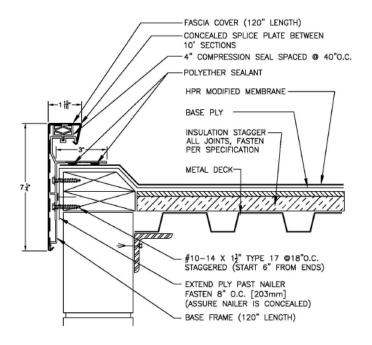
Note: 7.25" face size depicted in the detail above. 5.75", 8.75" and 10.25" face sizes also available. For all sizes, the fascia extends 2.25" above the roof edge or wood nailers.
