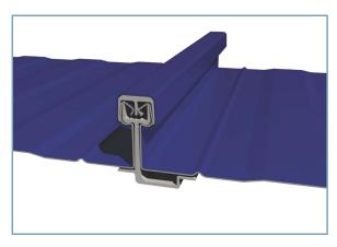
Garland's newest generation of industry-leading, high-performance, structural standing seam roof system boasts a 2-1/16-inch high vertical seam with an extruded aluminum clip and top rail system that provides outstanding wind uplift performance.
